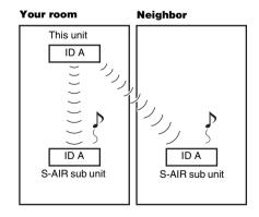
After pairing, sound transmission is established between the paired unit and S-AIR sub unit(s) only.
